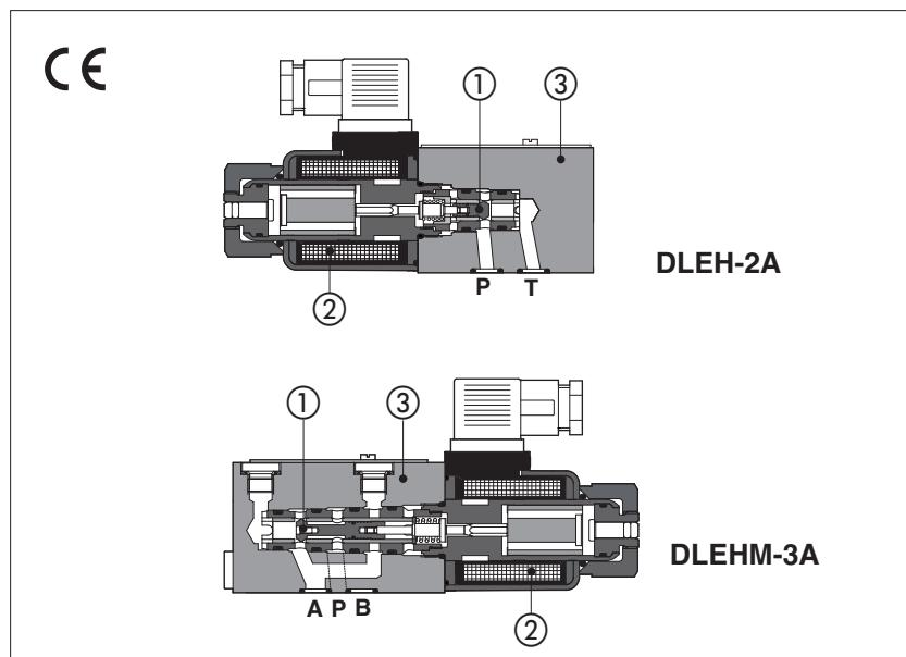
Poppet type ① direct operated valves, designed for applications in oil hydraulic systems with leak free requirements.
