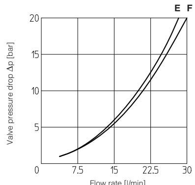
**8 OPERATING LIMITS** based on mineral oil ISO VG 46 at 50°C
